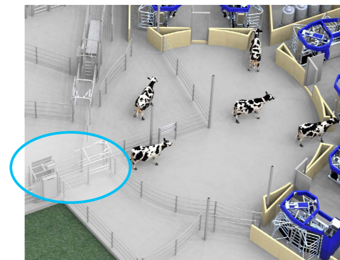
x1 additional SSG to accommodate 'special needs' opportunities in VMS's - A dedicated VMS can be used for treatment animals, colostrum. VMS's equipped with OCCs can do true cell count if required.
