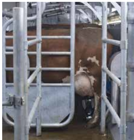
Entrance gate pushes last cow gently into milking position
