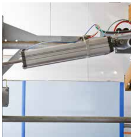
Duplex cylinder for front exit and indexing
