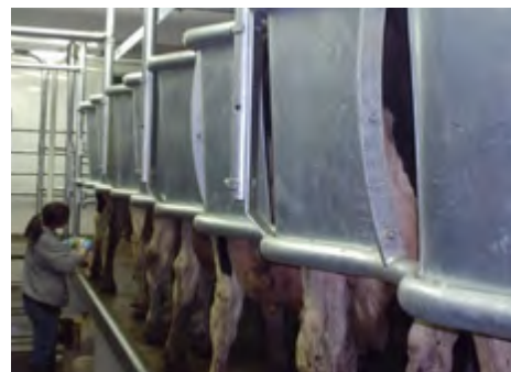
Excellent milker comfort, angled rumprail assemblies in Galvanized or optional Stainless Steel.
